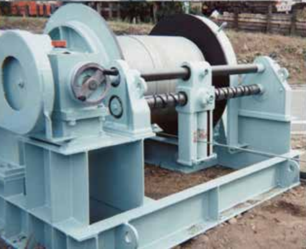
Antarctic Research "Electric winch MAW-1100 for deep ice coring system" for the 36th Japanese Antarctic Research Expedition
